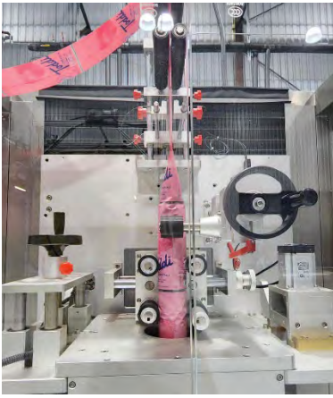
Special equipment required for the ready-to-drink line includes an apparatus that suctions the labels around the bottle
